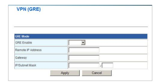
**GRE Enable:** Enable/Disable the VPN function for the FWT WIFI AP USB x 4.
